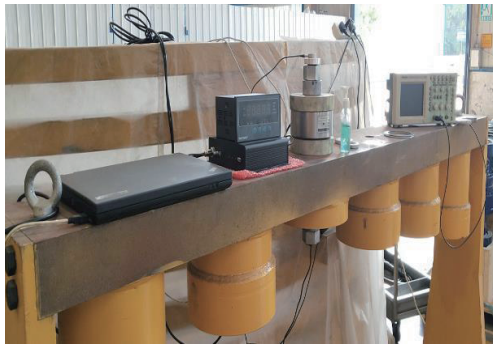
图1 螺栓轴向应力超声测量系统原理框图与测试现场 Fig. 1 Principle block diagram and test photo of ultrasonic measurement system for axial stress in bolts
